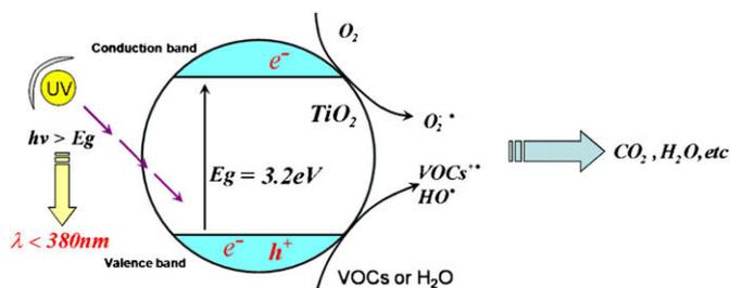
Fig. 1. Schematic of TiO<sub>2</sub> UV photocatalytic oxidation process of VOCs.
