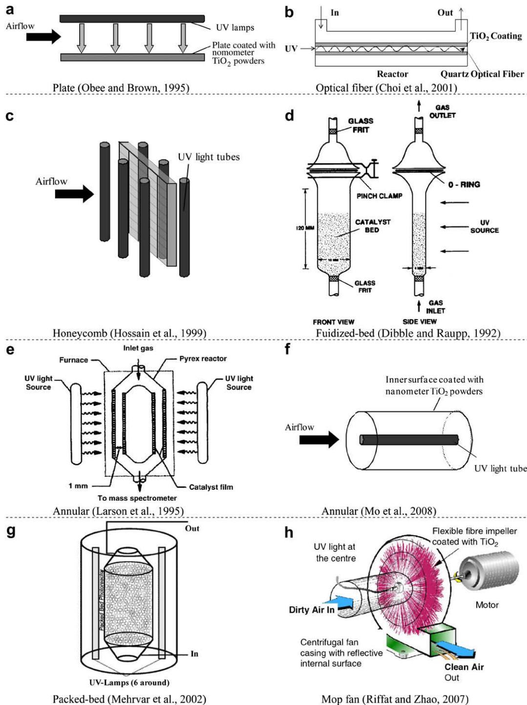
**Fig. 4.** Schematic of various PCO reactors. (a) Plate (Obee and Brown, 1995); (b) Optical fiber (Choi et al., 2001); (c) Honeycomb (Hossain et al., 1999); (d) Fluidized-bed (Dibble and Raupp, 1992); (e) Annular (Larson et al., 1995); (f) Annular (Mo et al., 2008); (g) Packed-bed (Mehrvar et al., 2002); (h) Mop fan (Riffat and Zhao, 2007).
