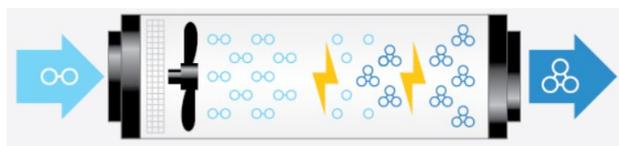
**Figure 5.** Visualisation of how a corona discharge ozone generator operates (Ozone solutions. 2021). <https://ozonesolutions.com/blog/what-is-ozone/>
